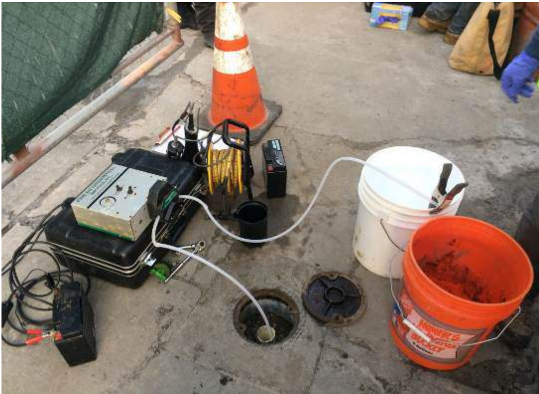
Photograph 108: View of the post-injection groundwater sampling set-up at the off-Site monitoring well SMW-1.
